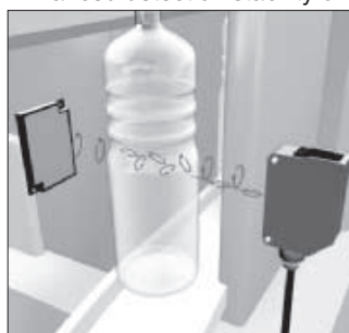
Utilisation of double reflection effect in PET for higher detection stability (PET optimised models)
